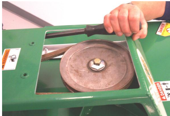
Adjusting Blade Drive Belt Tension
